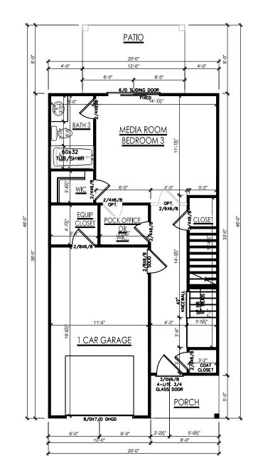
FIRST FLOOR PLAN 'AKAMATSU' SCALE: 1/8"=1'-0" ON 11x17, 1/4"=1'-0" ON 22x34
