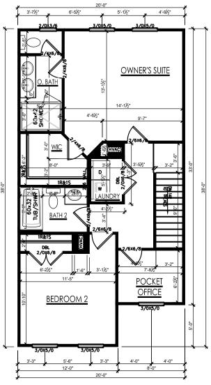
THIRD FLOOR PLAN 'AKAMATSU' SCALE: 1/8"=1'-0" ON 11x17, 1/4"=1'-0" ON 22x34
