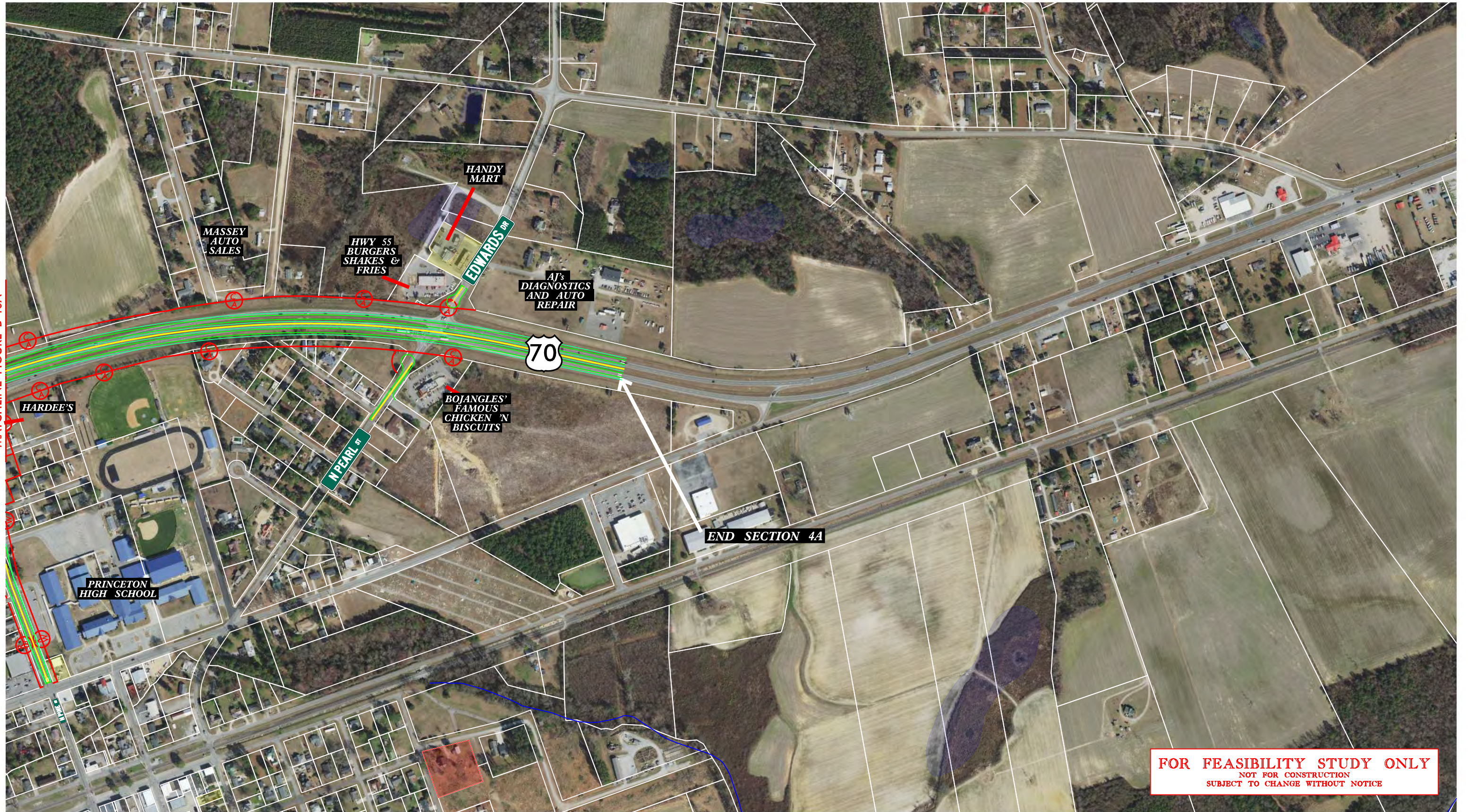
FIGURE B-11A CONCEPTUAL ROADWAY PLAN ALTERNATE 1
