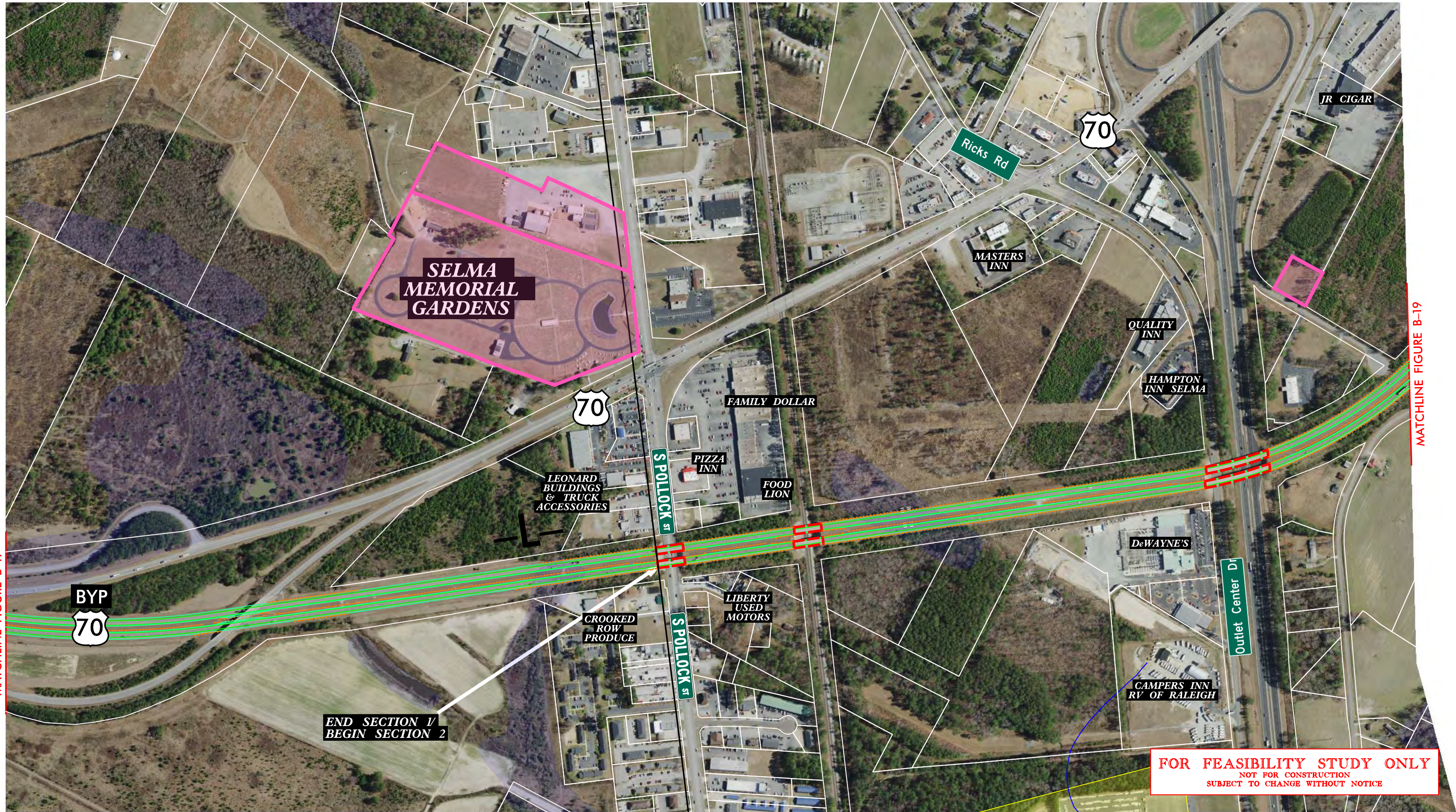
FIGURE B-18 CONCEPTUAL ROADWAY PLAN ALTERNATE 2
