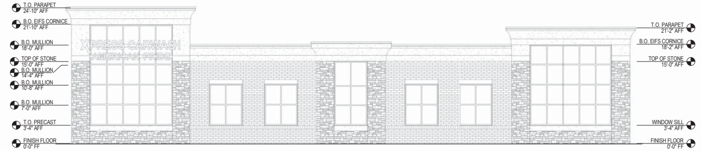
1 FRONT (EAST) ELEVATION 1/8" = 1'-0"
