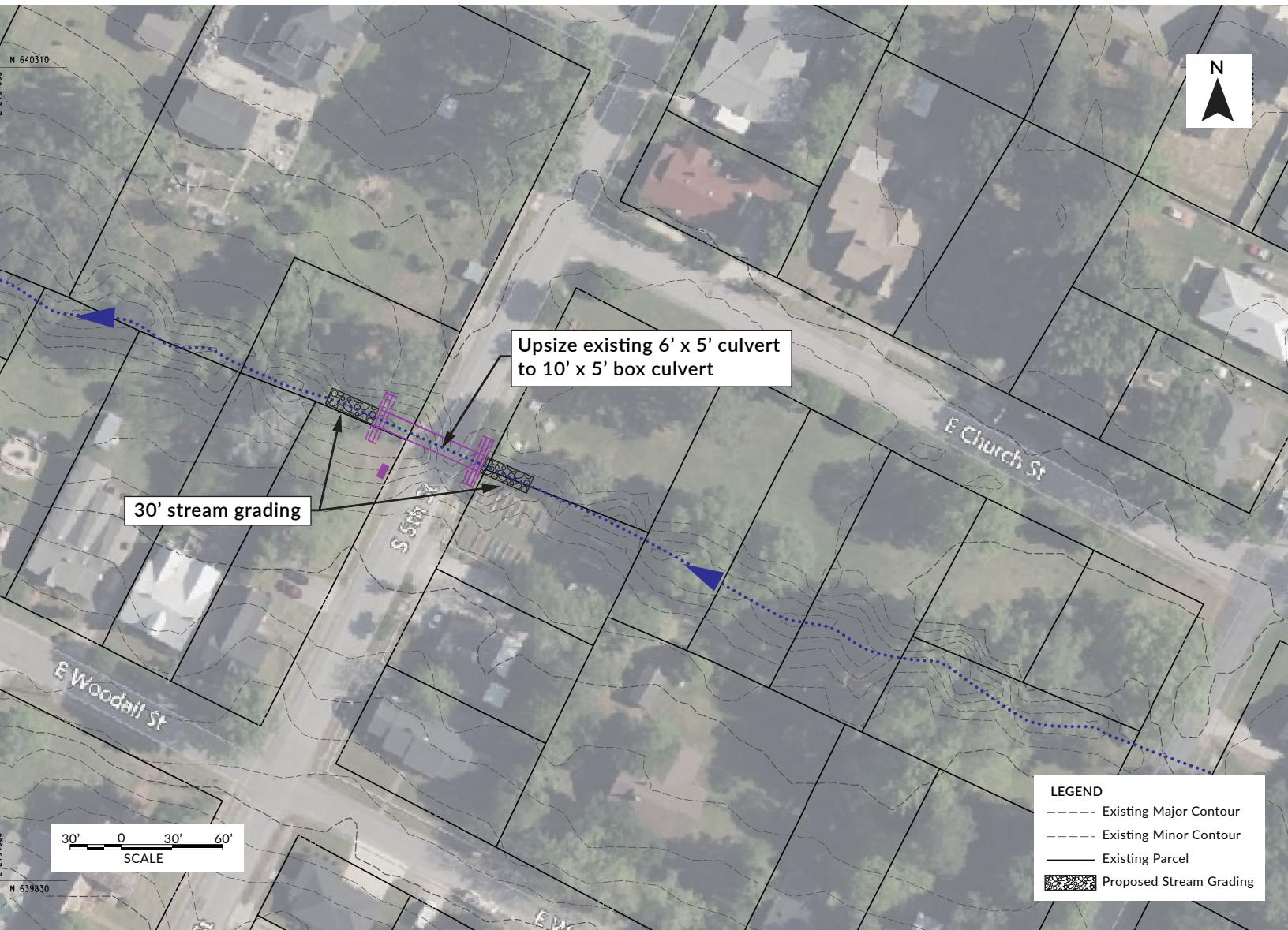
This proposed project would replace the existing 6' x 5' culvert with a 10' x 5' concrete box culvert to improve conveyance capacity. Upstream and downstream headwalls will be placed along with tie-in grading upstream and downstream to cleanly connect the new crossing into the existing stream. Further design will consider utility crossings, private property impacts, and connections to the stream.
